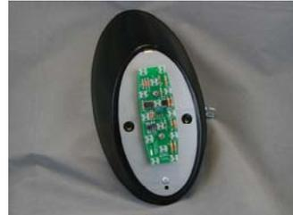
7. Remove the light divider from the taillight lens.
