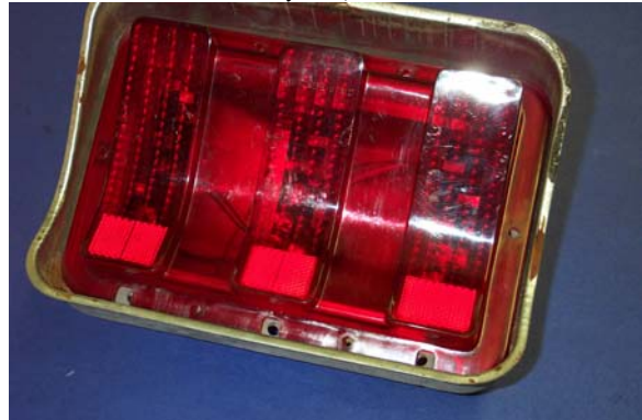
Finally, place the lens and thick gasket (not shown) on the assembly before placing it in the car.
