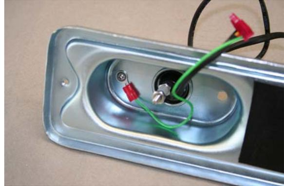
After connecting the wires to the truck, re-install the taillight housing into the truck. Note the green ground wire is attached to one of the mounting holes. Very important!
