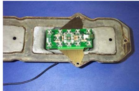
*Photo(left housing) shows correct LED placement. Note how the LED is centered in the stamped depression of the housing.*
