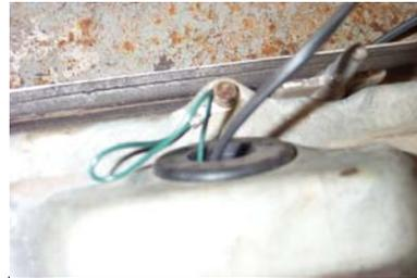
*Note the green ground wire attachment as well as the correct installation on the wire grommet in the outermost light.*
