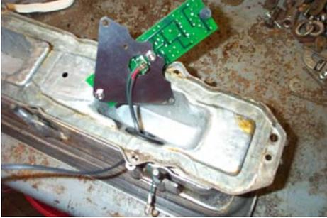
9. Place the gasket (new preferred) in the housing on top of the stainless LED bracket.
